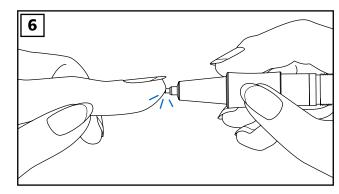
6) Push the refill all the way to the stop in. The Kaweco EMR insert is now ready for use.
