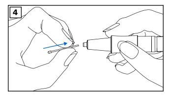
4) Take a new refill and position it infront of the Kaweco EMR insert opening. Be aware to slide the refill into the insert with the thinner end ahead.
